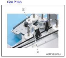
2. Remove the C-clip [1], and remove the horizontal transport clutch 1 [2].
