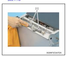
Using a soft cloth dampened with alcohol, wipe the transport roller [1] clean of dirt. Blank Page
