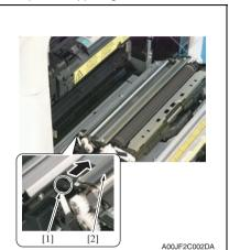
2. Pushing the hook [1], remove the paper dust remover [2].
