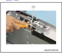
Using a soft cloth dampened with alcohol, wipe the tray 3 separation roller [1] clean of dirt.
