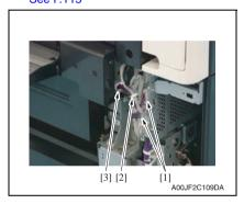
Disconnect two connectors [1], and remove the harness from the wire saddle [2] and the edge cover [3].
