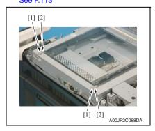
Remove each screw [1], and remove the original glass fixing bracket (near side/inmost side) [2].
