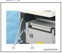
3. Remove three screws [1], and remove the rear left cover [2].
