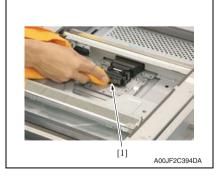
Using a soft cloth dampened with alcohol, wipe the lens [1] clean of dirt.
