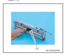
3. Using a soft cloth dampened with alcohol, wipe the roller [1].
