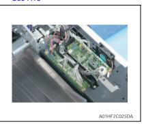
Disconnect all the fifteen connectors from the DF control board.
