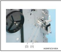
6. Remove the E-ring [1] on the rear side to remove the driving pulley [2].
