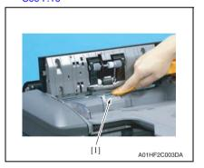
2. Wet a cloth with alcohol, and use it to wipe up the separation roller [1].
