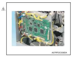
Remove all sixteen connectors (For FS-517/FS-518) or all seventeen connectors (For FS-608) from the FNS control board.
