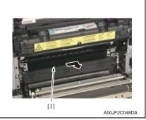
Slide the image transfer entrance guide [1] towards the back of the main body and remove it.
