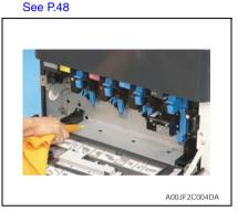
Wipe the areas around the waste toner collecting port clean of spilled toner and dirt using a soft cloth dampened with water or alcohol.
