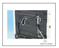
5. Disconnect the connector [1], and remove the duplex unit.
