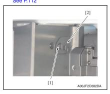
2. Remove the screw [1], and remove the cover [2].
