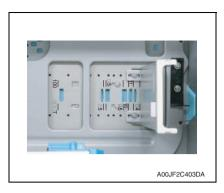
Align the paper guide plate (rear) with the marking on the bottom and secure it with four screws
